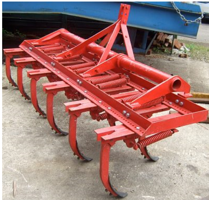
Tractor drawn cultivator- spring loaded tines
