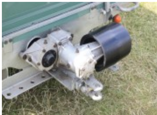
Belt pulley connected to tractor PTO
