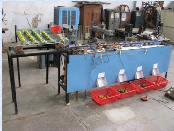
Plate 3.5 Orange grading (weight basis) machine in operation
