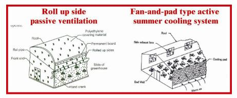
prevailing wind and rain (Fig.8). During the periods of excessive heat, it may be necessary to roll the sides up almost to the top. Passive ventilation can also be accomplished by
