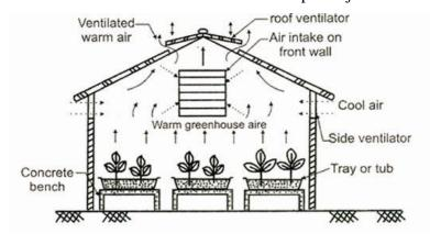
the greenhouse. The ventilators on the roof as well as those on the side wall accounts, each about
