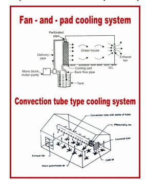
cooling the air everywhere. As this system does not wet the foliage, there is less scope for disease and pest attack. The plants stay dry throughout the process. This system is equally useful for seed germination and propagation since it eliminates the need for a mist system.
